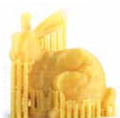
^ 3D printed rabbit with conventional support material
